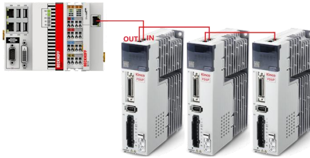
Figure 3-2 BECKHOFF CX5020 connecting drives
