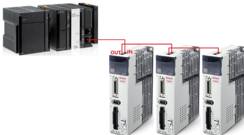
Figure 3-3 Omron NJ controller connecting drives
